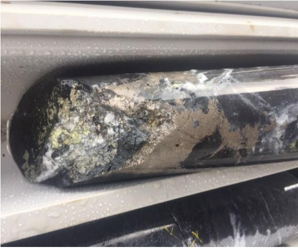
Image 6. Pyrrhotite-chalcopyrite in KB19DD004.
