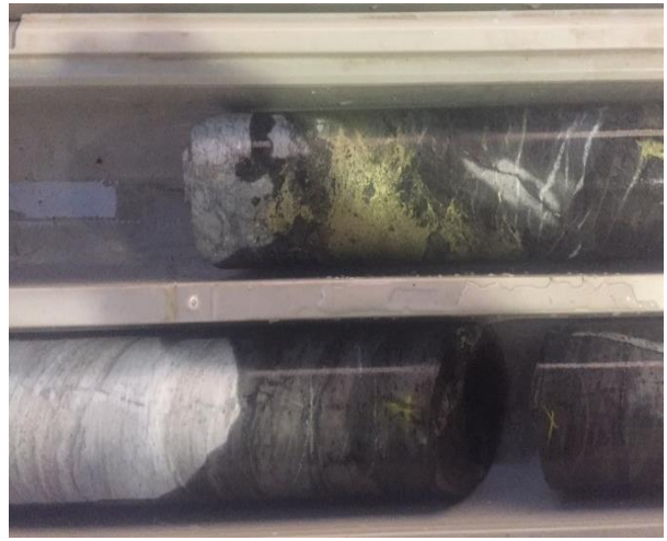
Image 7. Chalcopyrite within hole KB19DD004.
