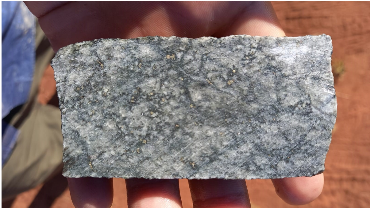
Figure 1. Bastion Prospect drill core photo from PLDD0005, 174.4m, 1.1 g/t gold hosted by disseminated sulphides in an intrusion.
