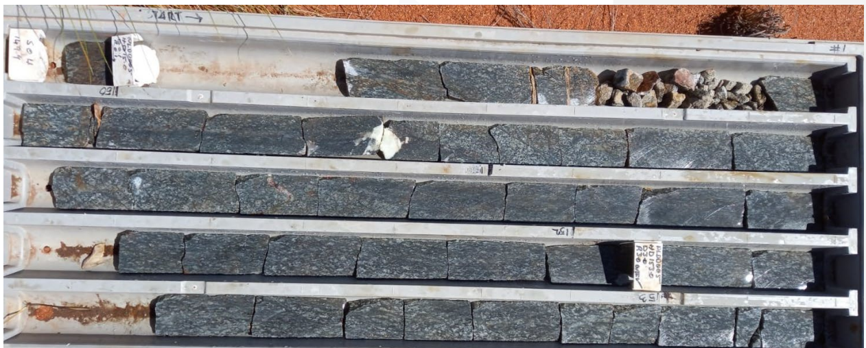
Figure 6. Bastion Prospect drill core photo from PLDD0005, 153.4m, 3.2 g/t gold hosted by disseminated sulphides in a strongly altered intrusion.
