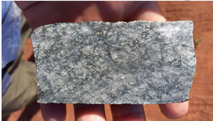
Figure 7. Bastion drill core photo from PLDD0005, 174.4m, 1.1 g/t gold hosted by disseminated sulphides in an intrusion.
