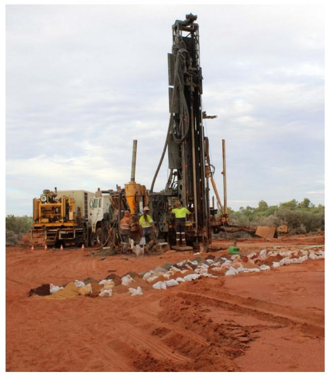
Image 1 / RC drill rig drilling sterilisation holes to the west of the existing heap leach pads
