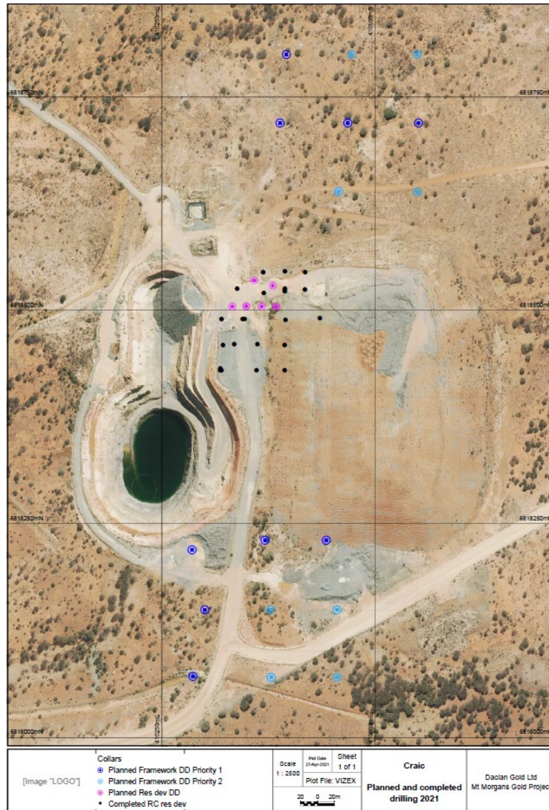
Figure 11: Craic drilling programs (black – completed resource development drilling; pink – additional resource infill drilling; dark blue – phase 1 extensional, light blue phase 2 extensional)
