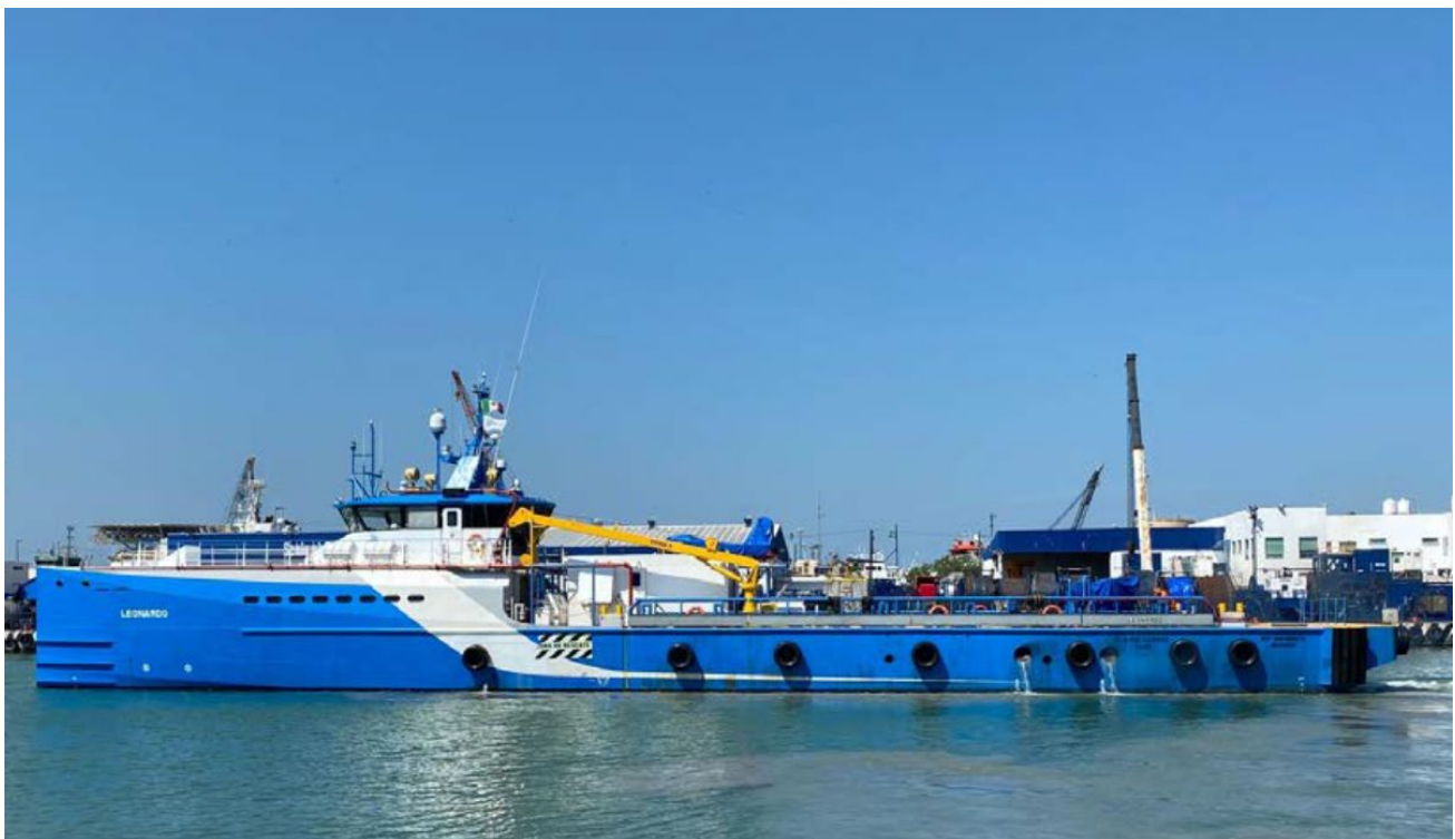
The MV Leonardo with the VG1000SD VEEM Gyro installed on the deck (below the yellow crane boom) ahead of sea trials.
