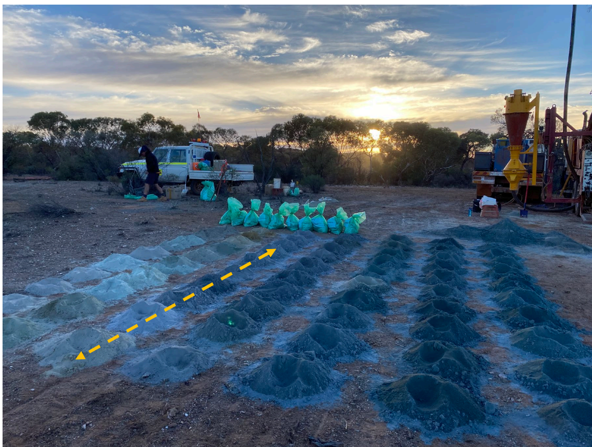
Image 1: IVRC001 completed with a 7m zone of sulphide alteration intersected (21m to 28m).
