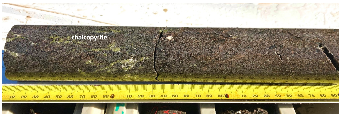
Figure 5 OBURCD025 interval 228m-228.2m showing altered diorite porphyry containing blebby chalcopyrite
