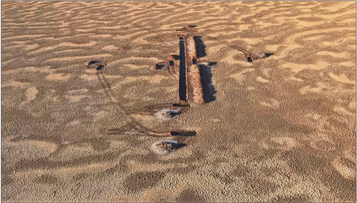
Figure 3: Lake Throssell - aerial view of a 100m long trial trench 01 with monitoring pits installed
