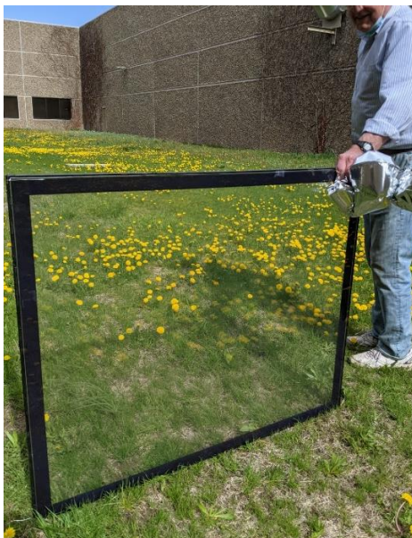
New double-glazed IGU prototype design (left). Looking through the new ClearVue double-glazed IGU design (right).
