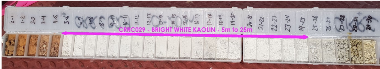
Figure 3: Drillhole CRRC029 with bright white kaolin from 5m to 25m (20m intercept)
