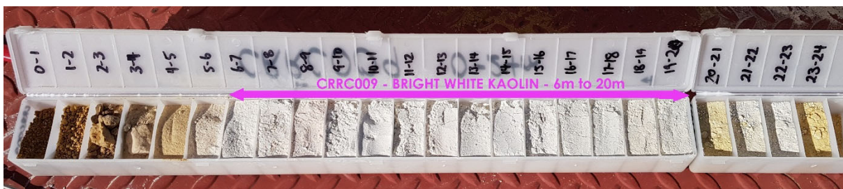
Figure 4: Drillhole CRRC009 with bright white kaolin from 6m to 20m (14m intercept)
