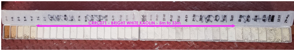
Figure 2: Drillhole CRRC071 with bright white kaolin from 5m to 33m (28m intercept)
