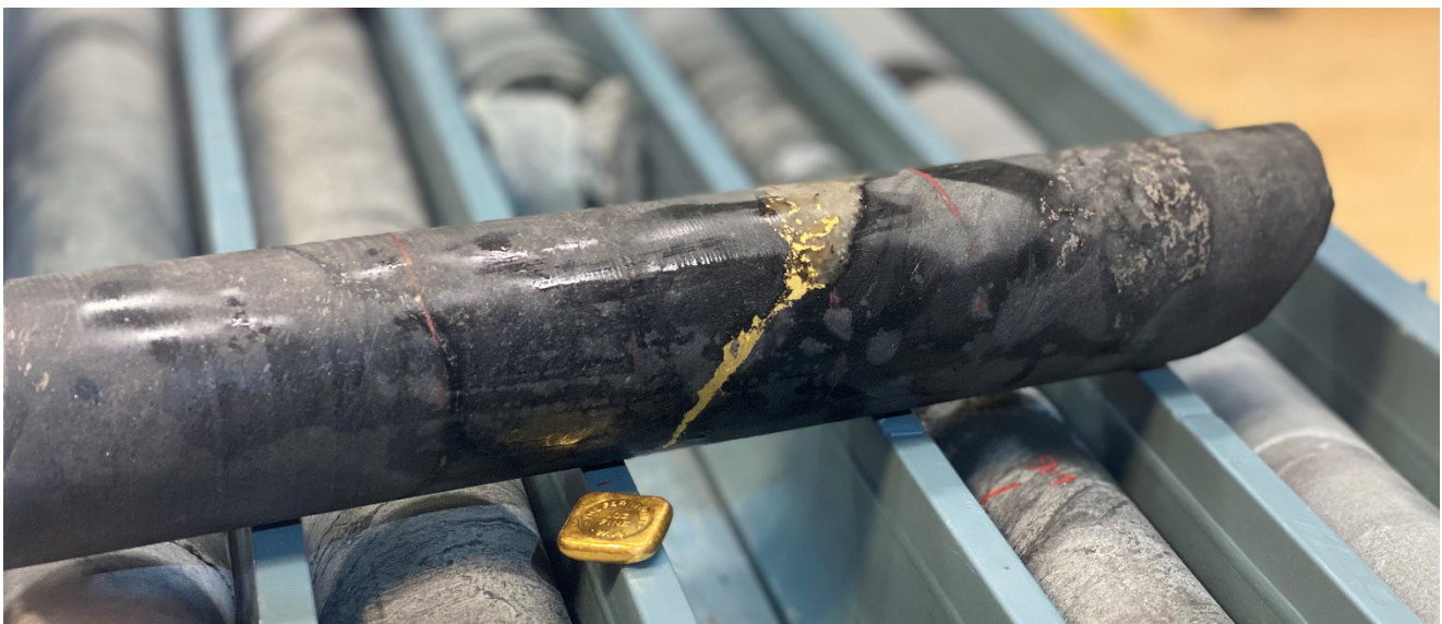
Figure 1. NQ core from diamond hole TCKD0003 showing the visible gold with a one ounce gold nugget for scale
