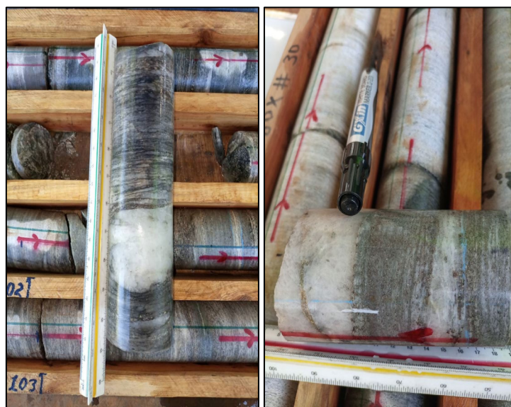
Figure 4 -Drill core from BBDD001 showing intervals of highly altered host rocks and quartz veining, both with significant visible sulphide mineralisation (pyrite, chalcopyrite, pyrrhotite). Left: ca. 101m Right: ca. 106m
