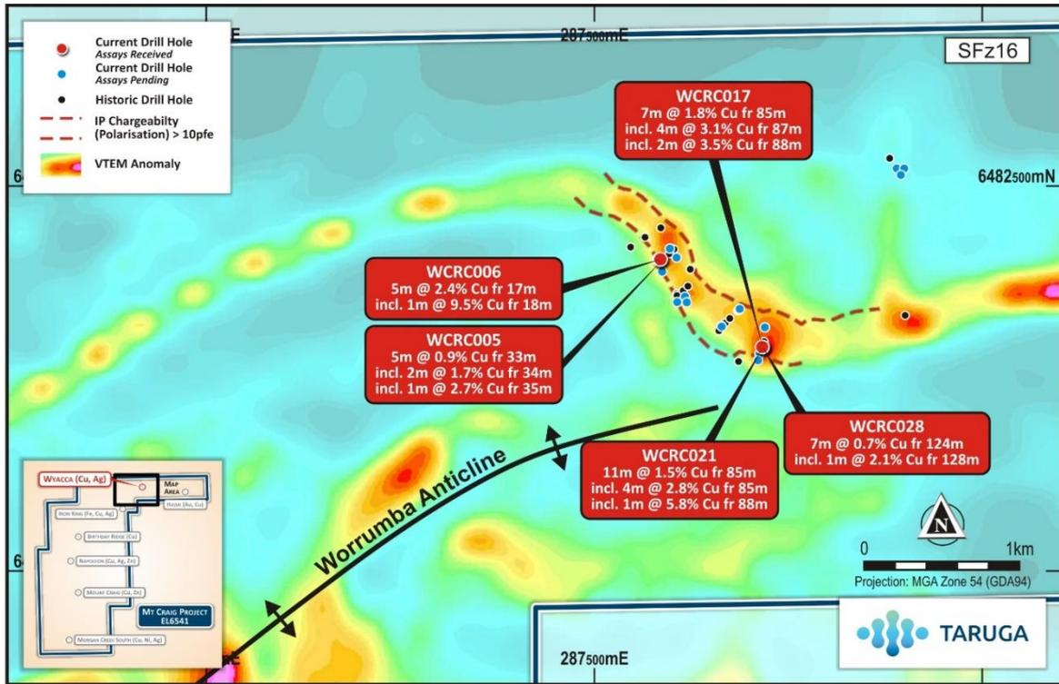
**Figure 1.** Image of the Vertical Component dB/dt Amplitude for Window 16 - 0.126 mSec, Highlighting 7km Early-Time VTEM Anomaly Coincident with IP Anomaly and Recent High-Grade Drill Results.
