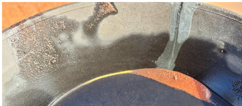
Photograph 1: Visible gold panned off from MNOAC 120 27-28m interval - 1m @ 162.5 g/t Au.
