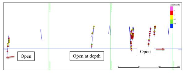
Figure 2: Leapfrog image: Section (looking east) showing previous drill holes at the Sawpit Reef area, also showing Au assays (>0.5ppm Au).
