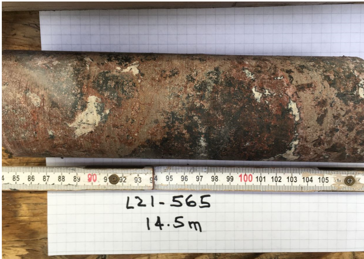
Figure 7 - Massive bastnaesite in drill hole L21-565
