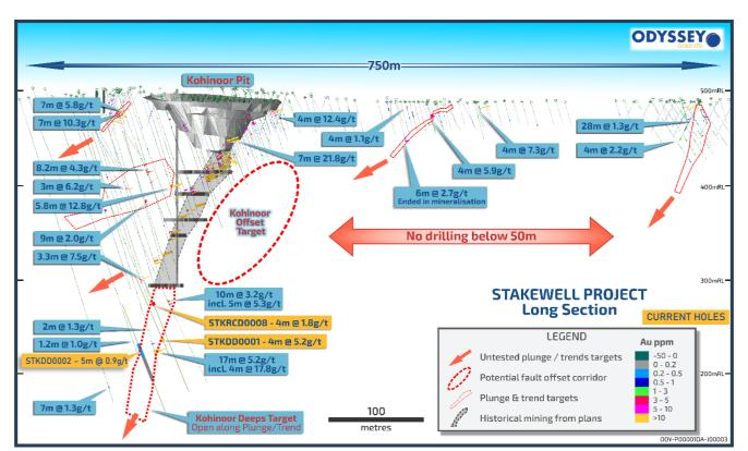
Figure 9. Stakewell targets showing recent diamond drilling.
