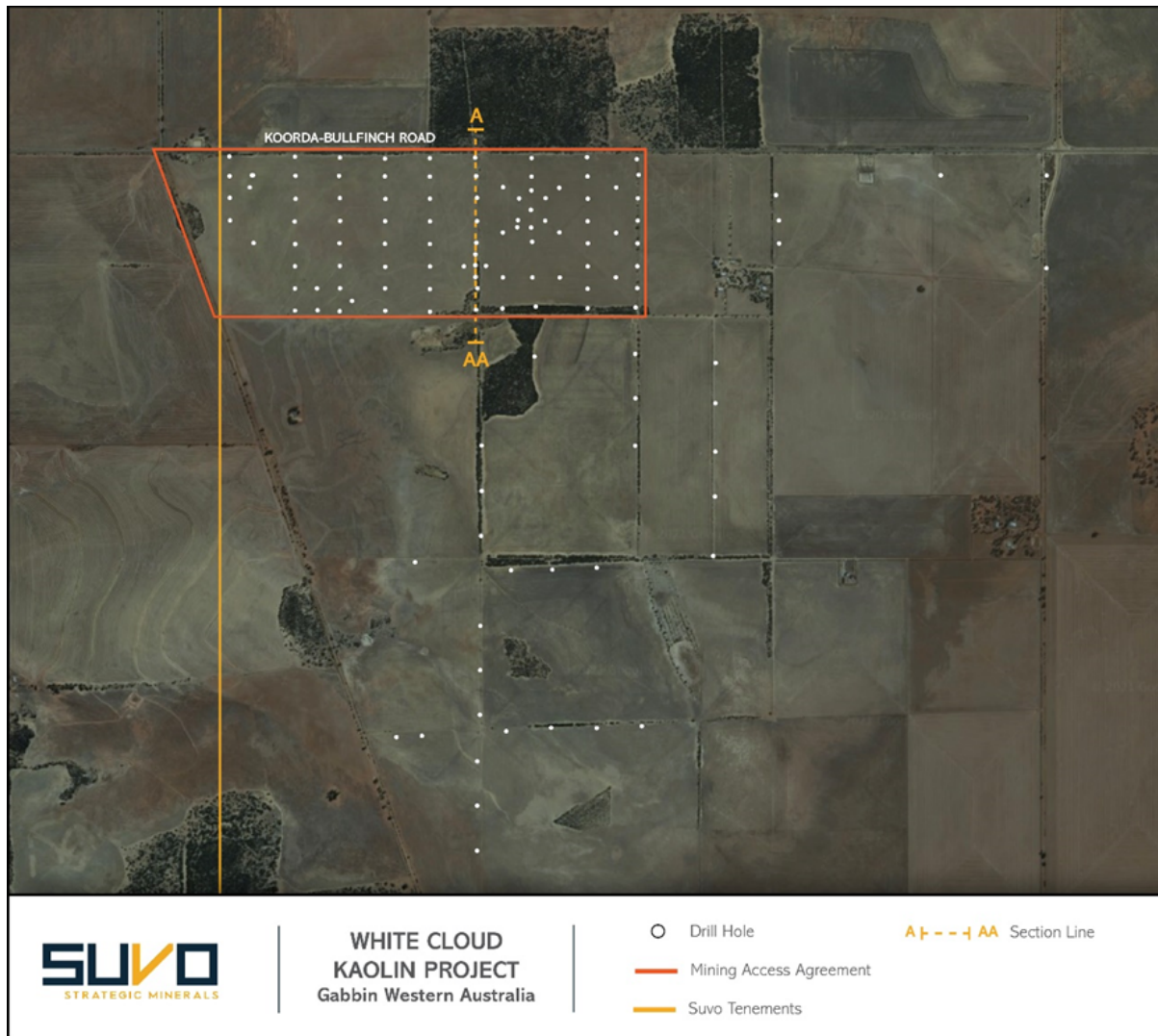
Figure 3 - Plan view of drill holes completed at the White Cloud Kaolin Project showing cross section
