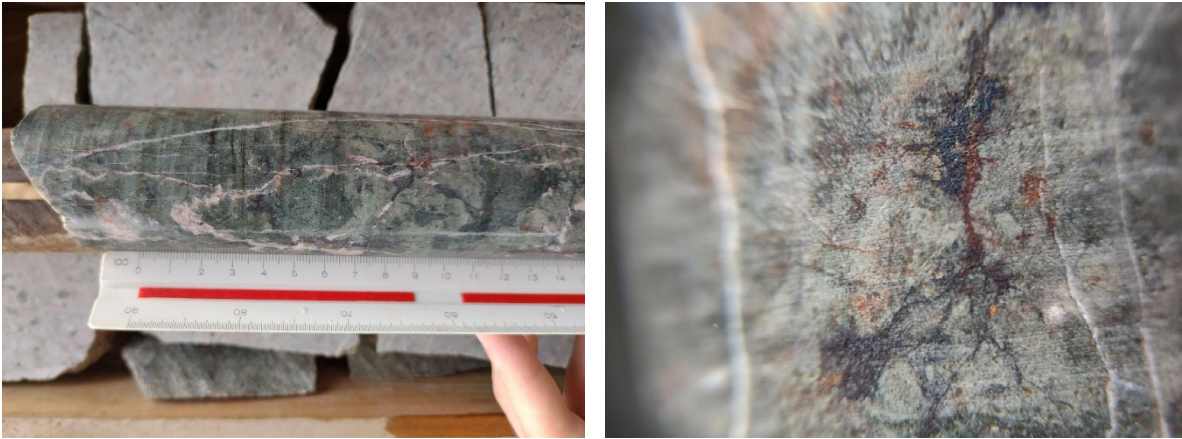
Figure 2: Breccias (with chalcopyrite and bornite infill) related to the Juruena Fault Corridor (from 830m). Field of view on RHS is approx. 4cm.
