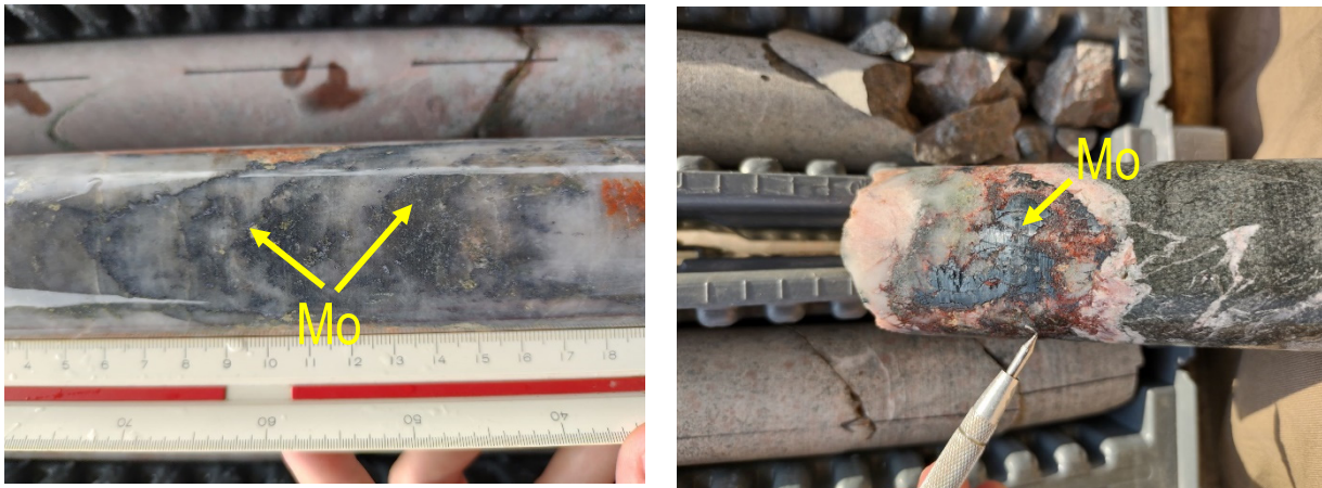
Figure 4: Quartz veins with high concentration of molybdenite are interpreted to track an increase in the temperature of the hydrothermal alteration and strong presence of Molybdenum in the system. (Mo = molybdenite)
