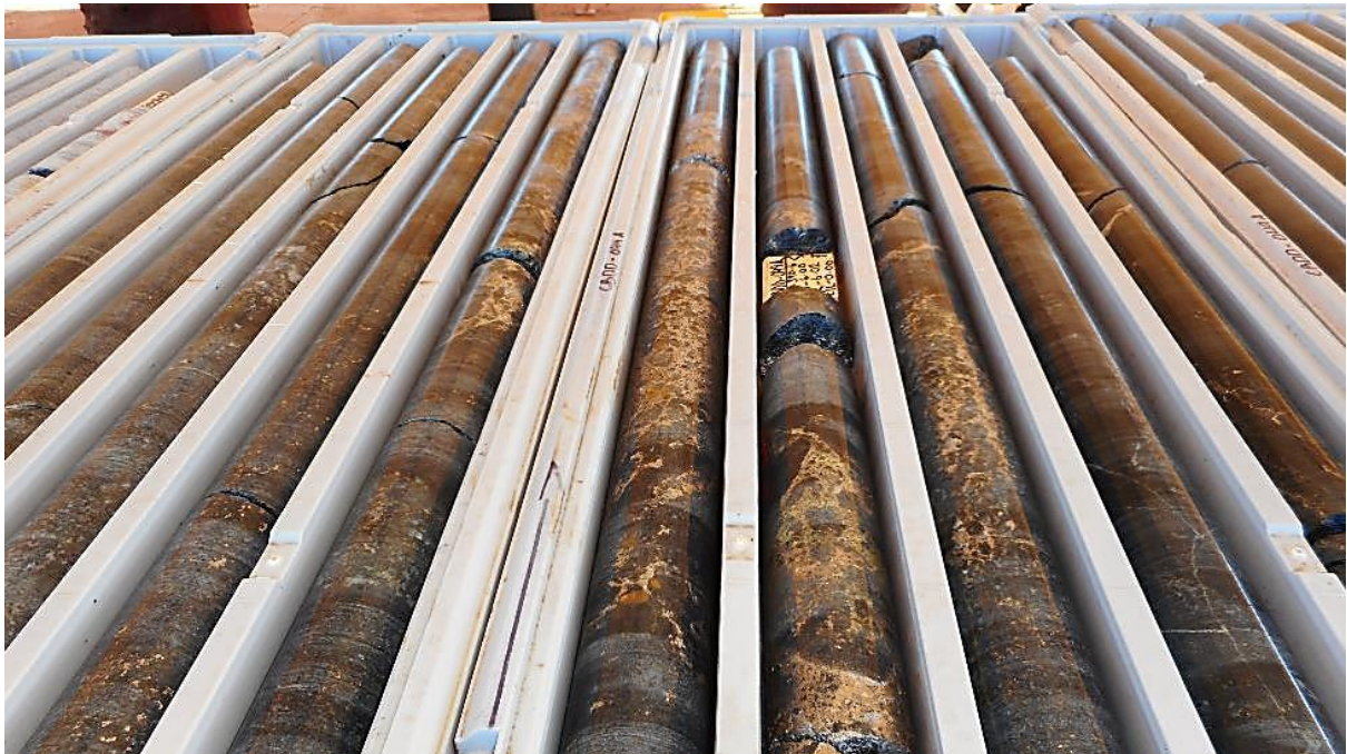
Figure 1: Massive and globular sulphide textures in CBDD049A at 388.5m on the T5 basal contact
