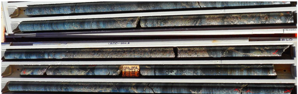
Figure 3: Photo showing the extent of the massive and globular sulphide zone in CBDD049A on the basal contact. The basalt contact (footwall) is half way along the last metre of core at the bottom of the photo.
