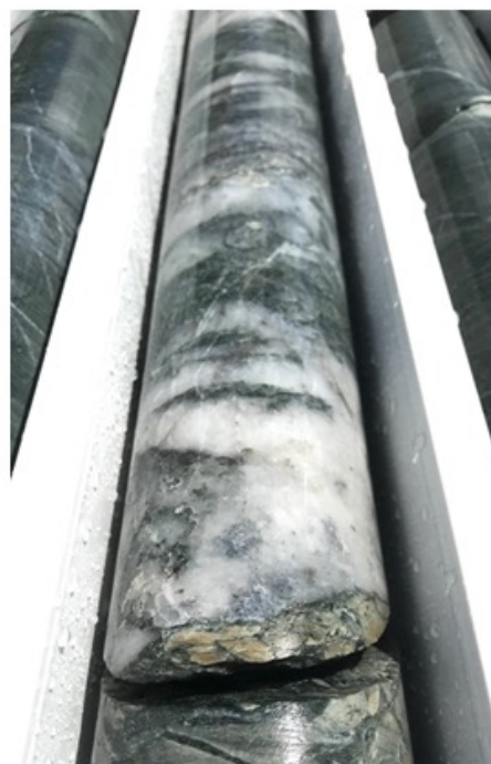
Photograph taken through a hand lens showing visible gold and Sailfish core from SFDD20-017.
