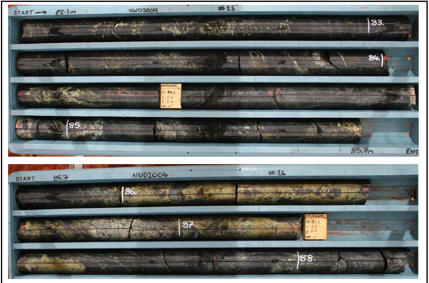
Image 1 | NWD2004: 82.1m to 88.0m; 5.9m @ 3.6% Cu chalcopyrite mineralisation, including 1.0m @ 10.9% Cu from 86.0m
