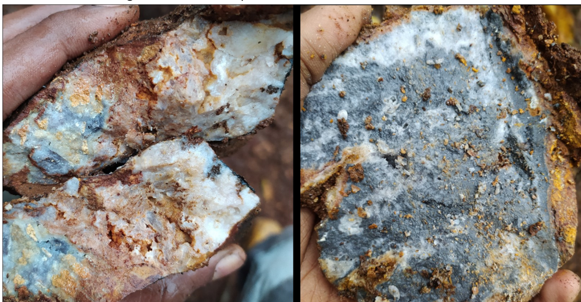
Photo 3: Quartz Sulfide Samples from Trench KC24 grading 1m @ 13.4g/t Gold + 32.5g/t Silver
