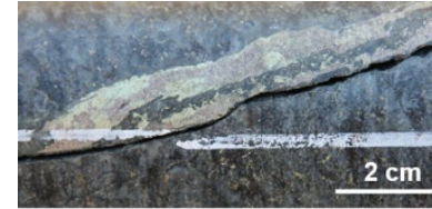
Late – stage pyrrhotite – chalcopyrite vein set with disseminated sulphide at 121.6m @ 121.6m
