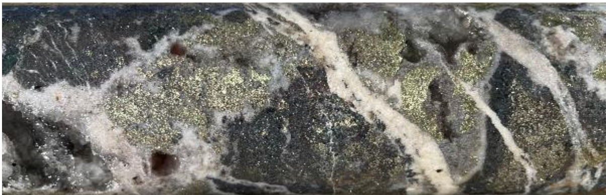
Vuggy chalcopyrite+pyrite veins in hematite+magnetite rock, cut by late carbonate veins. Large, perfectly terminated quartz crystals indicate slow crystallisation into open space. 537.2m.
