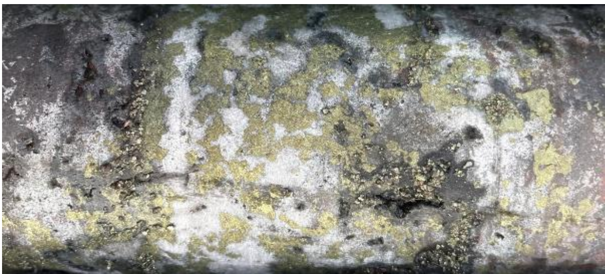
Intergrowth of chalcopryite+quartz/carbonate, partly replacing massive hematite with laths of hematite. 553m.
