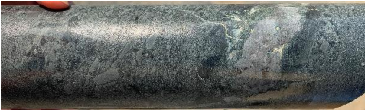
Silica altered serpentinite clast with patchy chalcopyrite in Alfa Breccia 1 at 494.3m.
