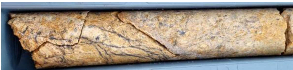
Serpentinite saprolite at 20.7m.
