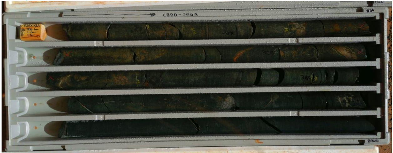
Figure 5: Massive sulphide breccia mineralisation within CBDD054A
