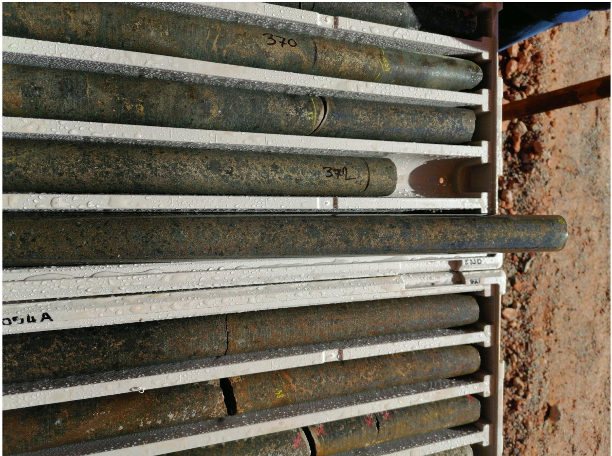
Figure 1: Massive-breccia and semi-massive nickel-copper-iron sulphides in CBDD054A at 369 to 377m. The total intersection ends at 388.49m downhole.
