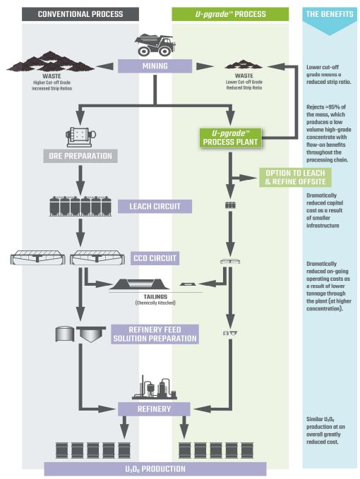
Using the *U-pgrade™* process could reduce process capital and operating costs by about 50%\*
