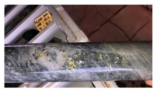
*Figure 5:* Chalcopyrite associated with quartz veining from 112.6m in drill hole BLDD002.
