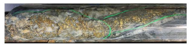
*Figure 3:* Vein chalcopyrite and pyrite from 32.7m in drill hole BLDD003.
