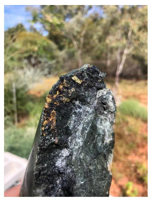
*Figure 2:* Vein and fracture-fill chalcopyrite and chalcocite from 23.5m in drill hole BLDD003.
