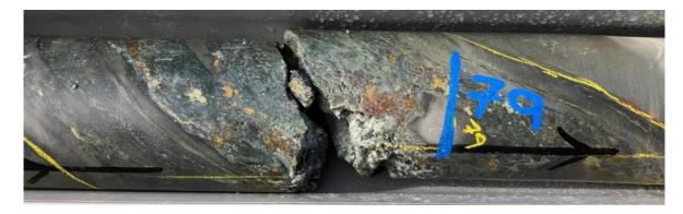
*Figure 6:* Vein and fracture-fill chalcopyrite and chalcocite from 78.9m in drill hole BLDD001.
