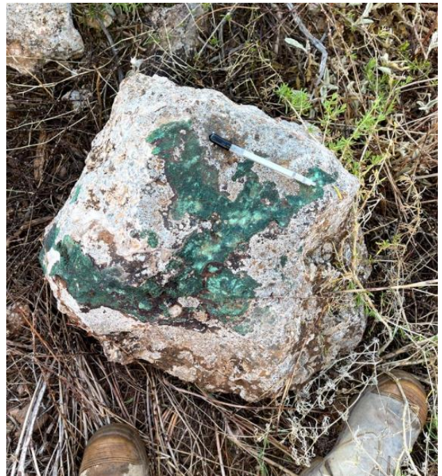
Figure 8 A (left) Rich Bornite, Chalcocite, Chalcopyrite and Malachite Mineralisation within Coarse Dolomite Breccias from the Worrumba 21 Mine Spoils; and Figure 8 B (right) Outcropping Gossan
