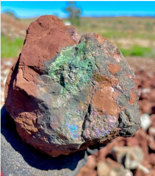
Figure 8 A (left) Rich Bornite, Chalcocite, Chalcopyrite and Malachite Mineralisation within Coarse Dolomite Breccias from the Worrumba 21 Mine Spoils; and Figure 8 B (right) Outcropping Gossan
