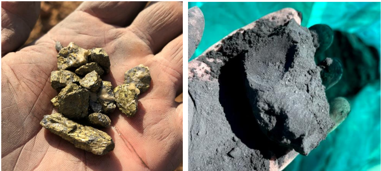
Figure 9 A (left) Rich Chalcopyrite Mineralisation (primary/hypogene zone) from RC Drill Chip from Drillhole WCRC021 (88-89m), which Graded 5.9% Cu , and 9 B (right) Rich Chalcocite Mineralisation in a Black Powder Unit (supergene zone) from Drillhole WCRC006 (18-19m) at Powder Hill, Grading 9.5% Cu .
