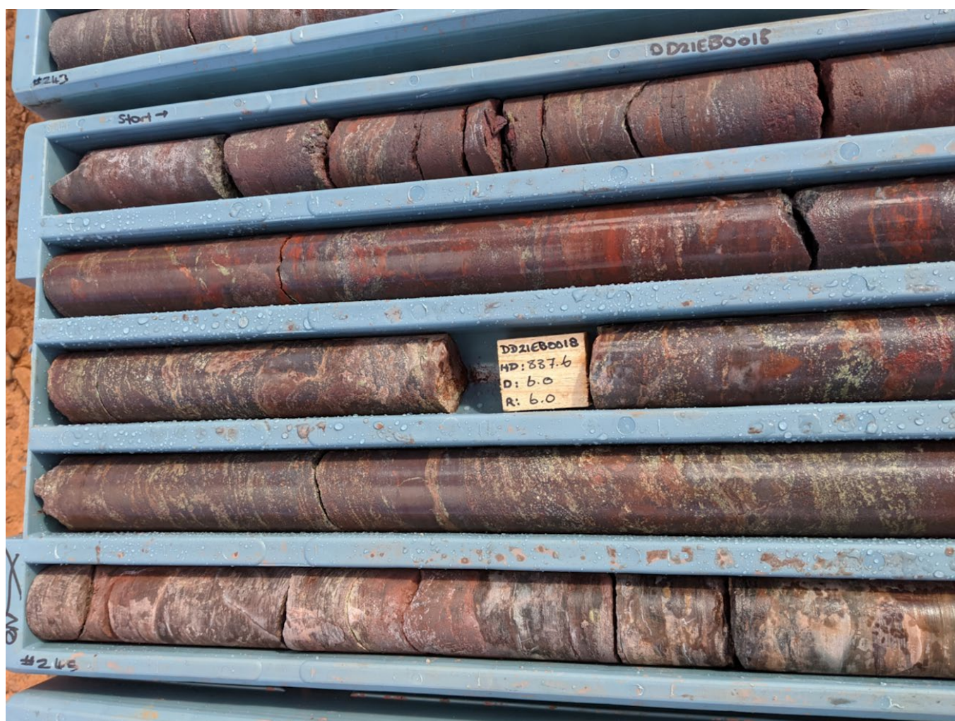
Figure 11 Typical alteration/copper sulphide pattern within the approx. 50m zone of copper sulphide mineralisation identified from approx. 797m. Chalcopyrite is the dominant copper sulphide, occurring generally parallel to remnant bedding of altered sediments, but also in small veinlets and blebs. Bornite is present only as fine disseminations in this section but is present in larger concentrations further down the hole. Note the intense patches of silica and chlorite alteration which occasionally dominate over haematite. Silica alteration becomes more intense with depth eventually dominating after approx. 850m.
