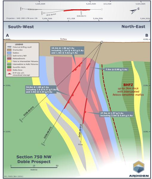
**Figure 5 – Cross Section A-B from Ardiden's Dobie Prospect.** For section location, refer to Figure 2 plan. For drillhole results, refer to ASX announcement 18 February 2020.
