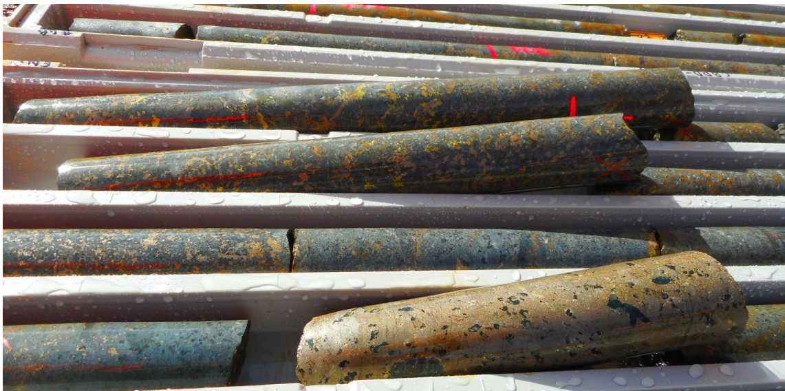
Figure 1a: Massive and globular nickel-copper-iron sulphide breccias in CBDD054B at 368m
