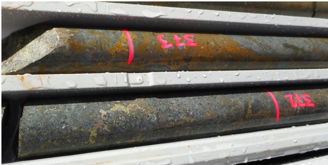
Figure 2b: Massive and globular nickel-copper-iron sulphide breccias in CBDD054B at 373m
