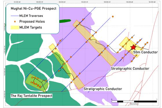
Figure 2 Preliminary MLEM conductor, stratigraphic targets, and planned tantalite drilling at The Raj, Mughal Prospect
