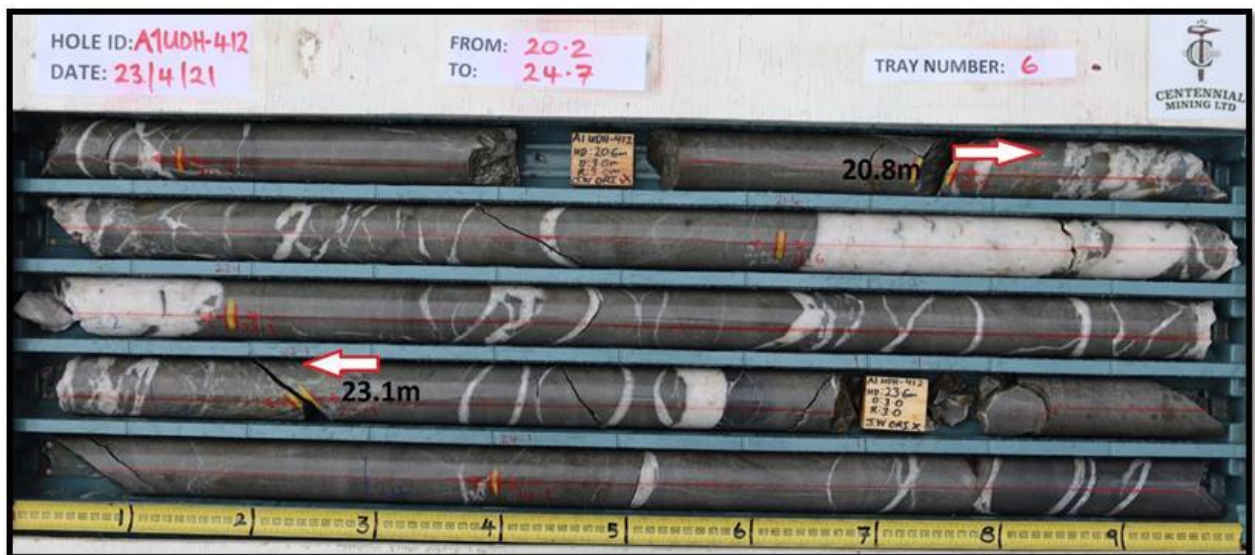
Image 2 - Gold mineralisation within sediment hosted quartz veins. 2.3m @ 11.63 g/t Au from 20.8m – 23.1m.
