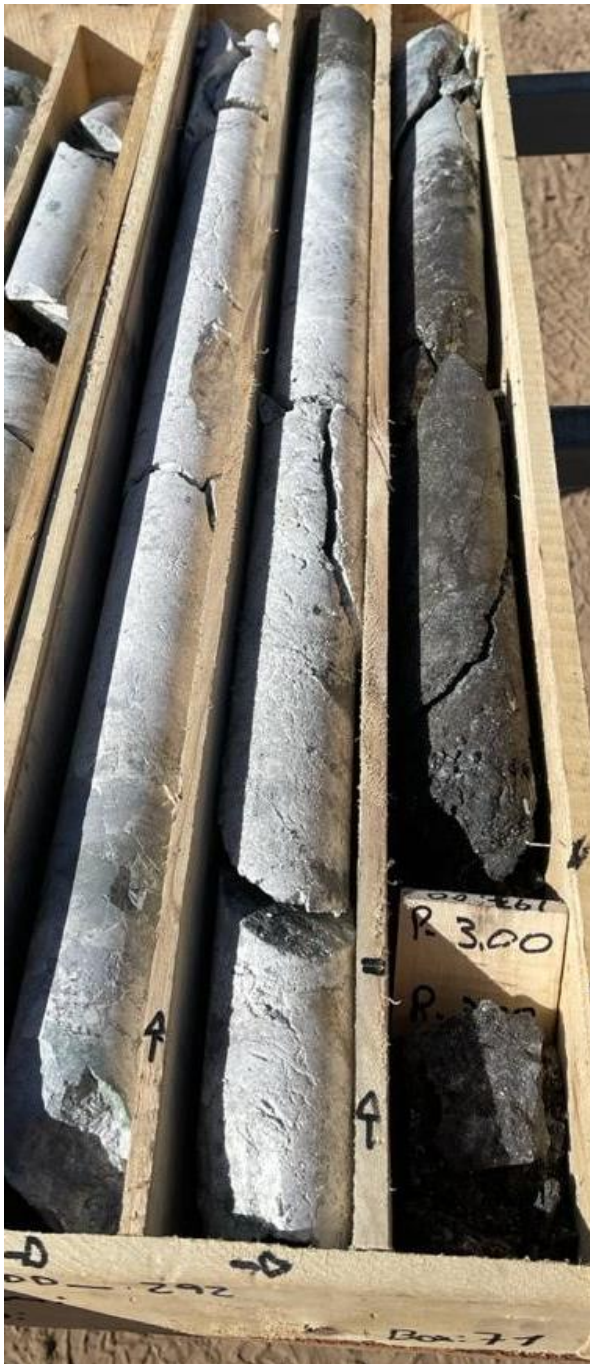
GNDD-292 - sulphide Interval 197-198m
