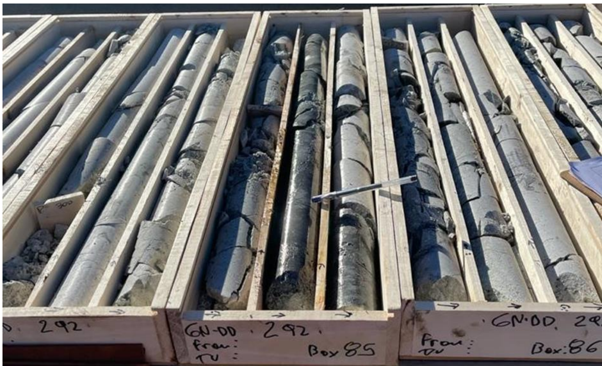
Photo 1 : GNDD-292 sulphide Interval 233 metres downhole (skarn alteration 15% pyrite 5% sphalerite)
