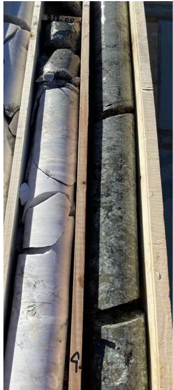
GNDD-292 - sulphide Interval 218-219m
