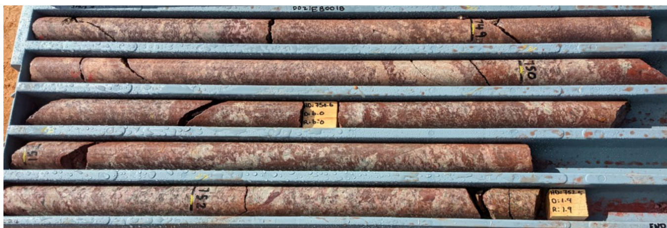
Figure 9 Haematite and chlorite altered Hiltaba suite granite. Chloritisation becomes stronger with depth.
