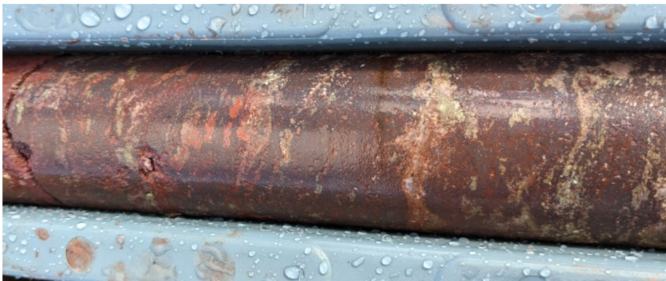
Figure 12 Closeup of drill core from approx. 838m showing texture of copper sulphides and alteration of host rock.
