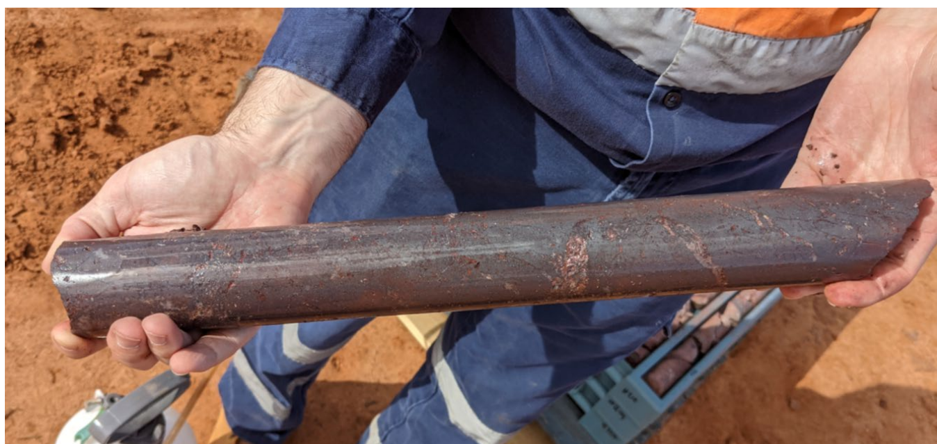
Figure 8 Near total replacement by haematisation of Wandearah Siltstone, close-up. Core starts at approx. 710.2m downhole. Alteration intensity is relatively typical of massive haematite cap overlying Hiltaba granite.
