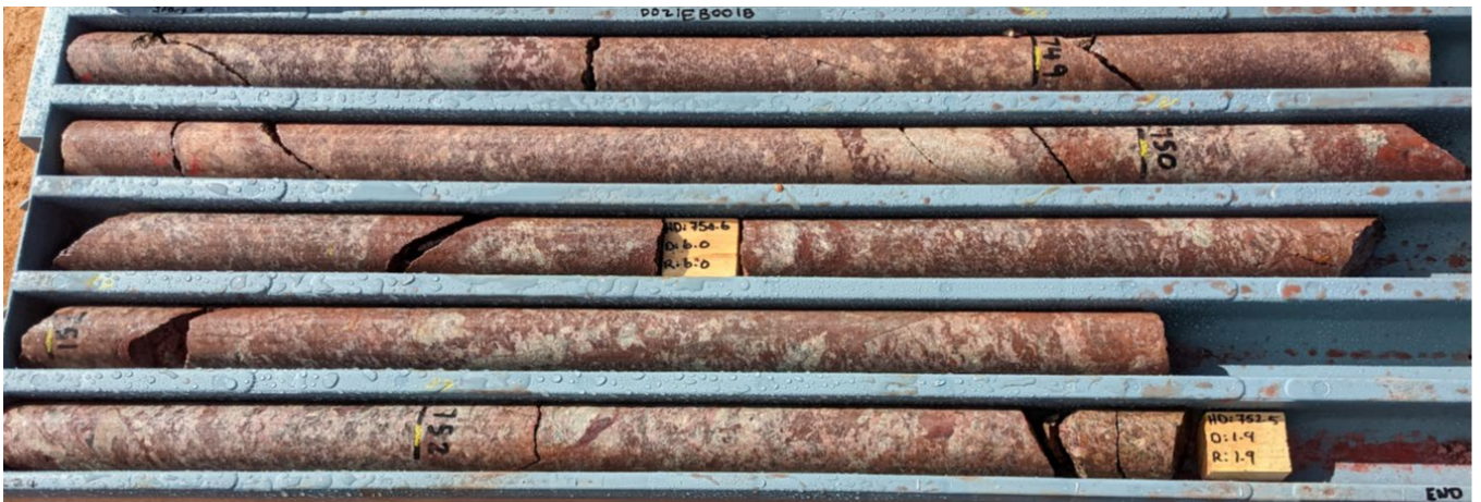
Figure 9 Haematite and chlorite altered Hiltaba suite granite. Chloritisation becomes stronger with depth.
