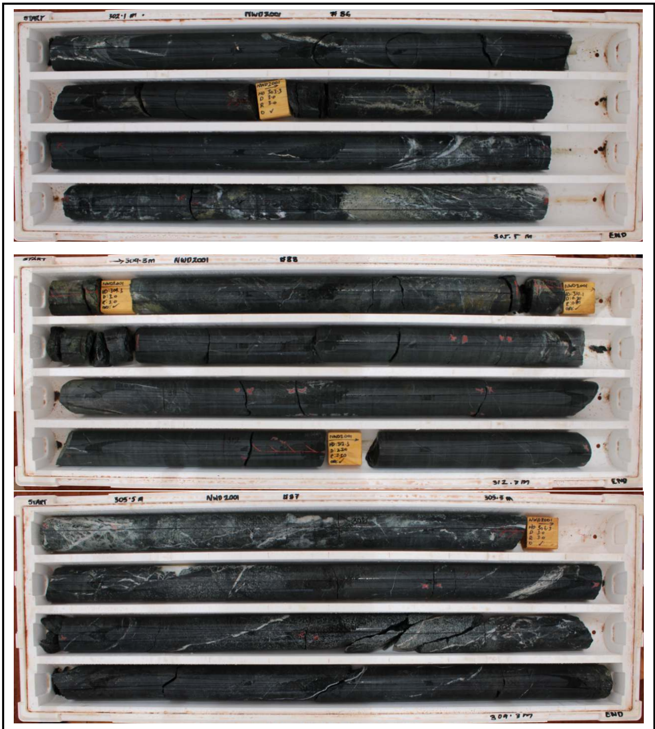
Image 1 | NWD2001: 303.0m to 312.0m; 9.0m @ 392 Ag g/t crackle breccia silver sulphide mineralisation, including 2.0m @ 1,470 Ag g/t from 306.0m.
