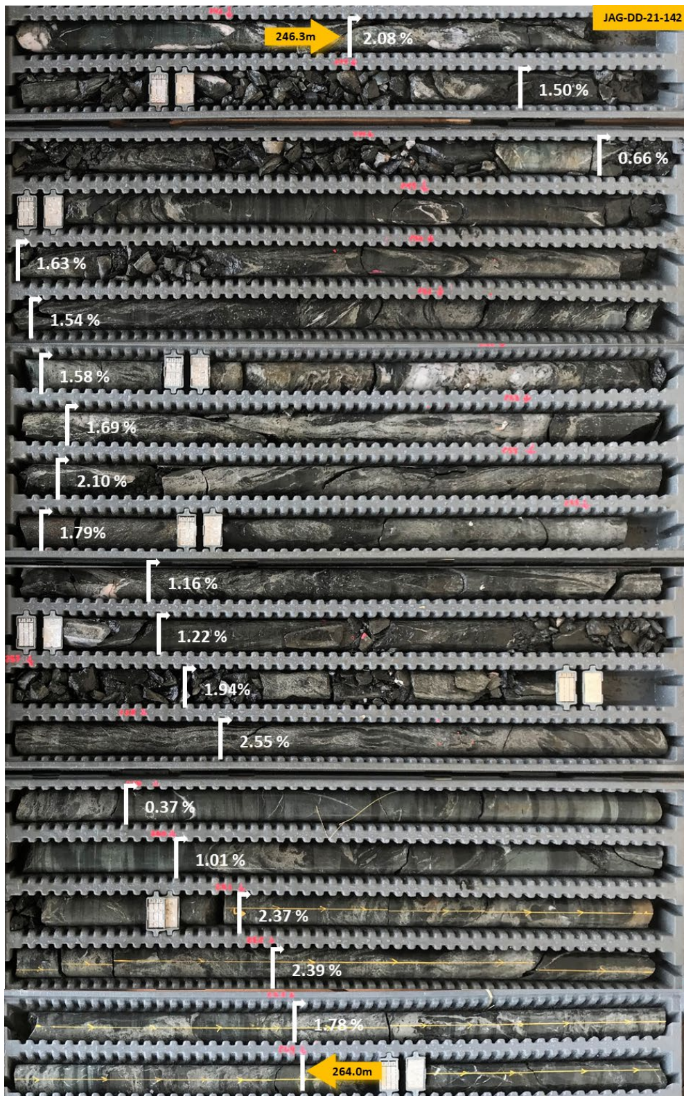
Figure 4 – Core photo from drill hole JAG-DD-21-142 (Jaguar Central); 246.3m to 264.0m down-hole: Disseminated, stringer to semi-massive sulphides (metallic bronze/yellow colour) with magnetite (black colour) mineralisation hosted in altered dacite. This interval returned: 17.7m at 1.62% Ni, 4.39% Zn, 0.10% Cu and 0.04% Co
