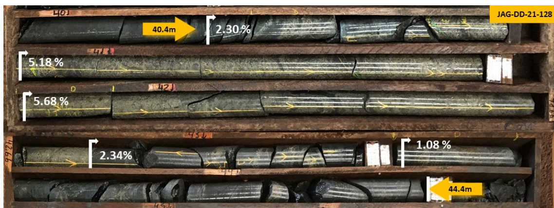
Figure 6 – Core photo from drill hole JAG-DD-21-128 (Jaguar West); 40.4m to 44.4m down-hole: Semi-massive sulphides (metallic bronze/yellow colour) with strong magnetite (black colour) mineralisation hosted in altered gneiss. This interval returned: 4.0m at 3.60% Ni, 0.03% Zn, 0.17% Cu and 0.08% Co
