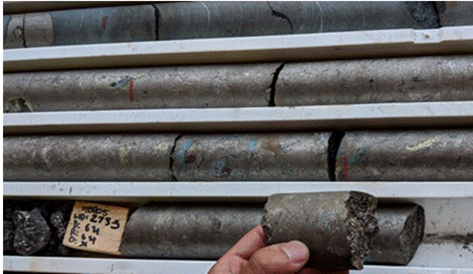
Figure Two | Massive Sulfides in TOR05 from drilling at the Thor “Julimar lookalike” Target
