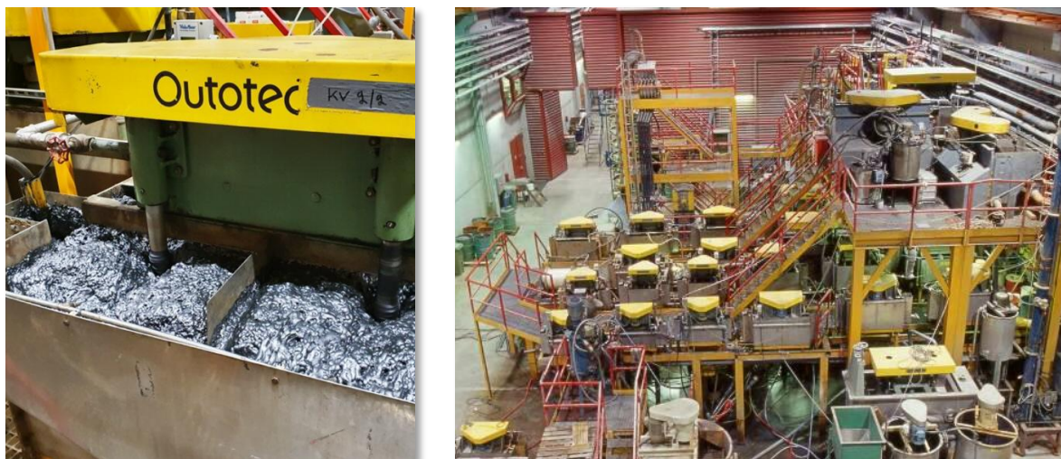
Figure 9 60 tonne bulk sample of Vittangi graphite ore being milled and concentrated at GTK, Finland.
