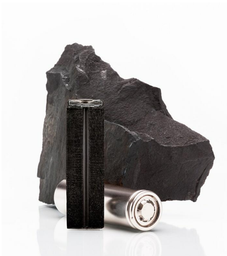
Figure 3 Vittangi graphite surface sample with 18650-size Li-ion batteries showing anode layers.
