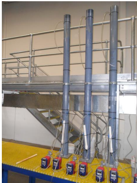
Figure 8 Commencement of 2021 60-day Column Leach Tests (CIT, RAS, SRE)
