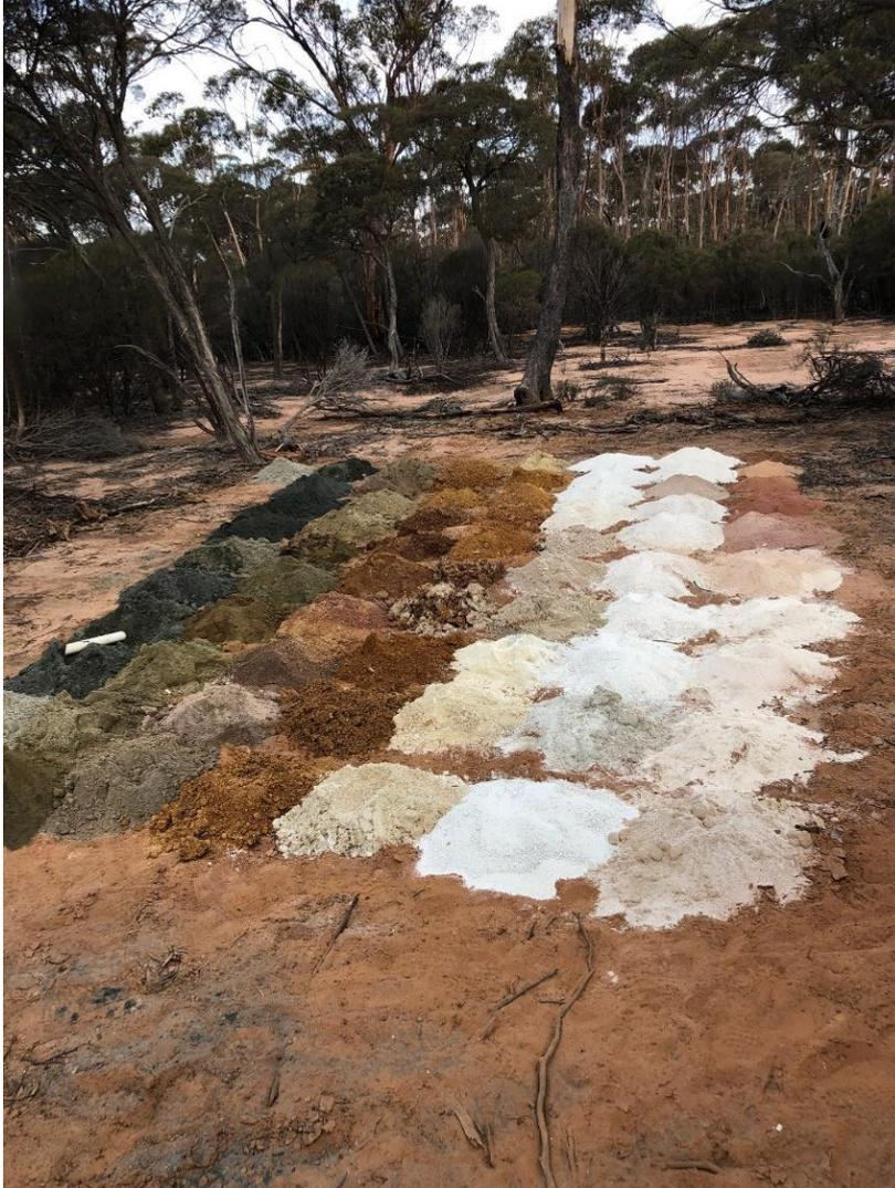
*Figure 2. Displaying RC drilling samples*
