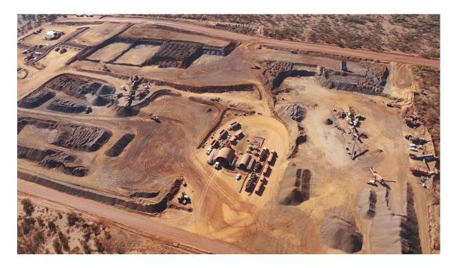
Figure 3: Stage 1 pit with recently cleared area for Stage 2 footprint – pit and waste dump
