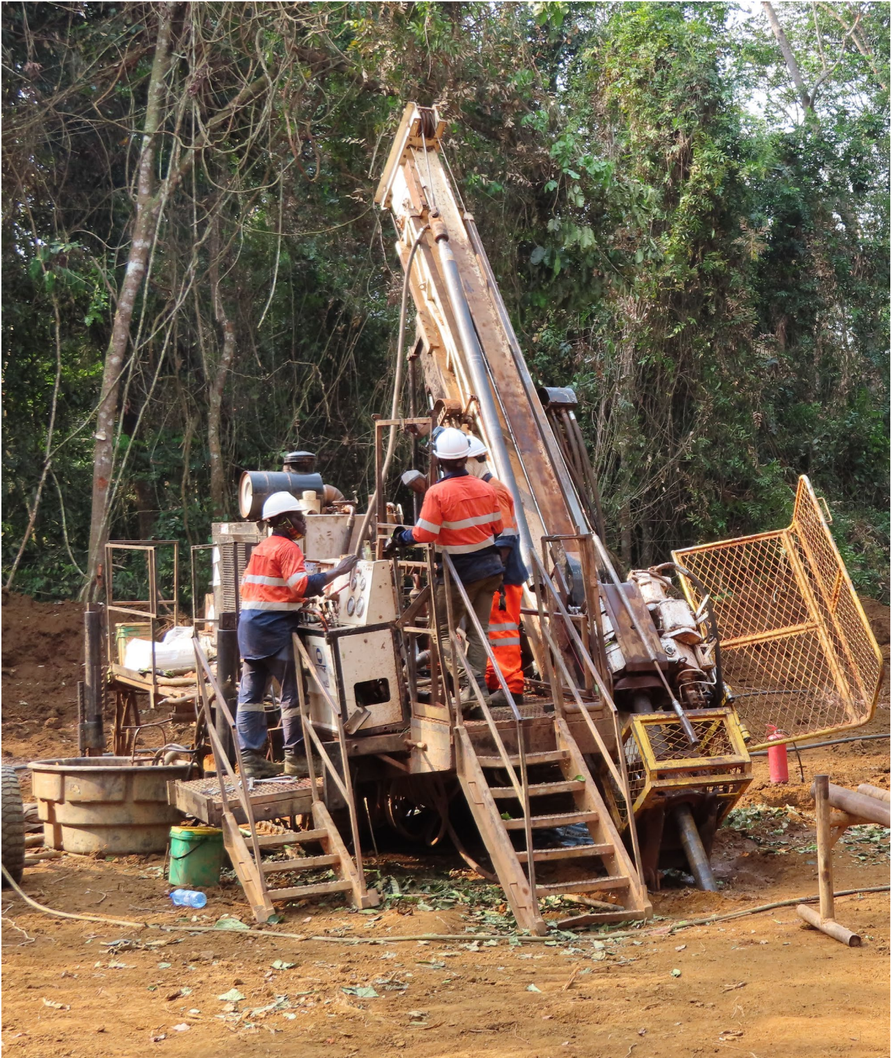
Figure 4: Diamond drilling at Bandjougoy prospect on 30 June 2021 (Drill Hole BWDDH0013, planned depth 125m)
