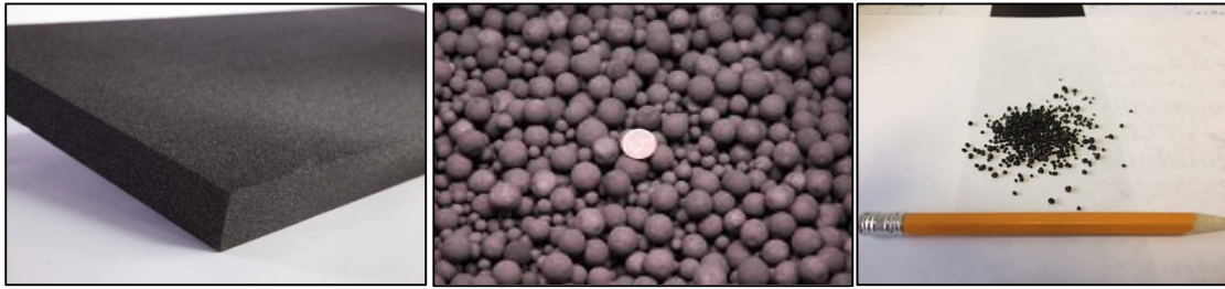
Carbon foam panel (left, 2x18x38 inches) and lightweight carbon foam aggregates - coarse and fine.
