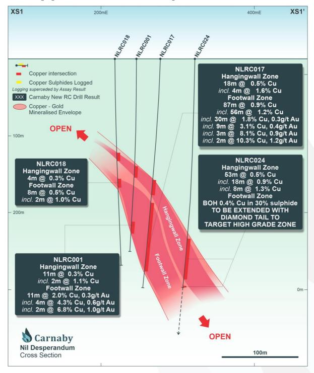
Figure 1. Nil Desperandum Drill Cross Section Showing New RC Drill Results.
