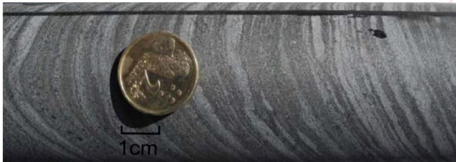
*BIF magnetite mineralisation in drill core from hole YS12DD017*
