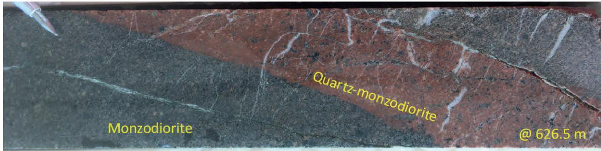
(a) Monzodiorite (grey) cut by orange-red quartz-monzodiorite at 626.5m down hole, in turn cut by quartz-carbonate veinlets (white).
