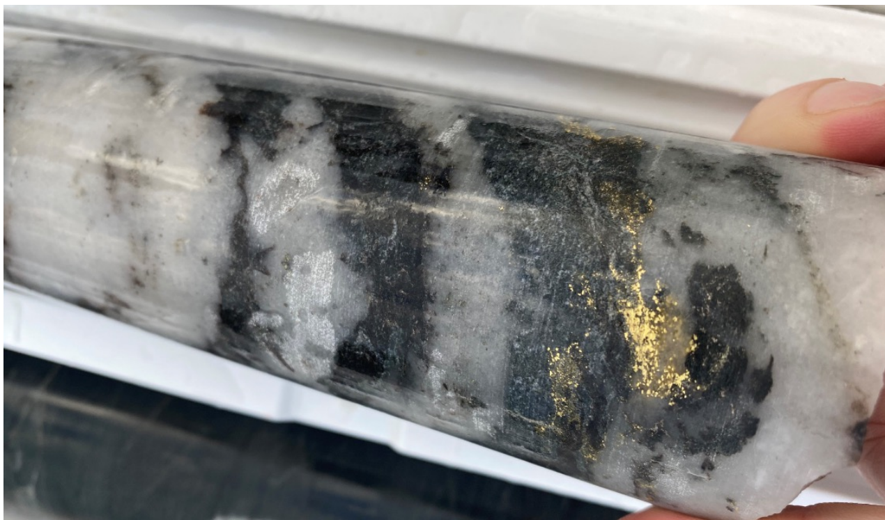
Section of interval from hole MARCD21_058 - 5.7 m @ 35.85 g/t Au inc. 1.4 m @ 141.57 g/t Au.
